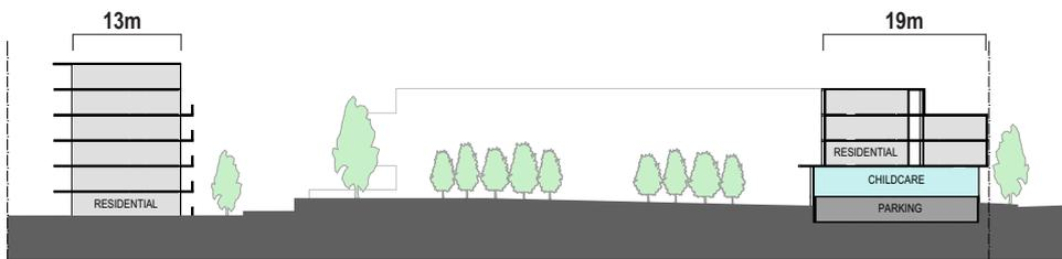
FIGURE 12. BUILDING DEPTH THROUGH BUILDING B & D
