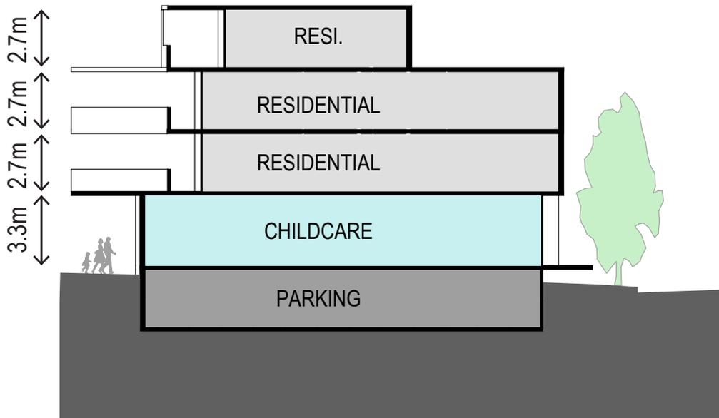
FIGURE 8. CEILING HEIGHTS SECTION THROUGH BUILDING D
