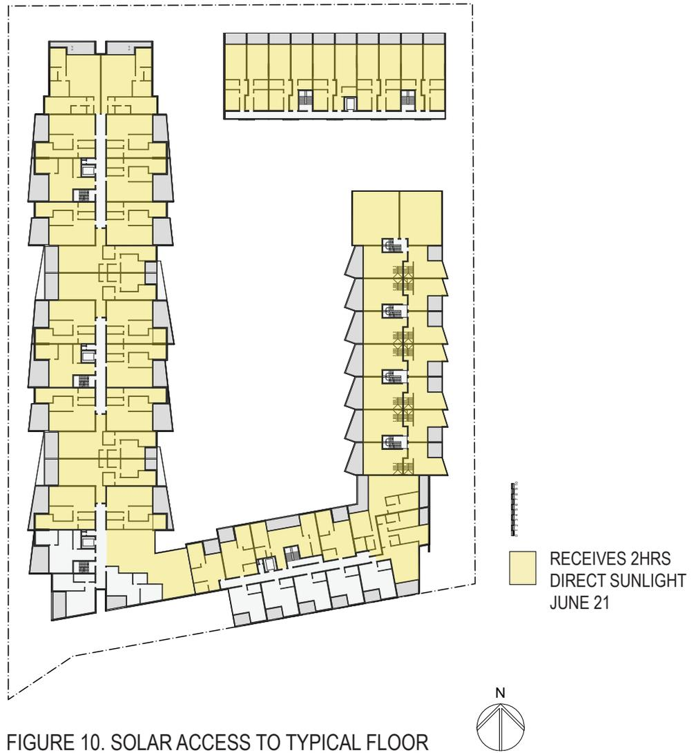
FIGURE 10. SOLAR ACCESS TO TYPICAL FLOOR
